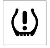
When a low tire pressure condition is detected, the TPMS will illuminate the low tire pressure warning symbol located on the instrument panel cluster.
