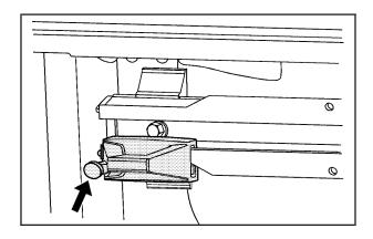
To adjust a tie-down, pull the locator pin out and move the tie-down to another location making sure the locator pin lines up with a locator hole on the rail. The tie-down pin may not be installed correctly if the pin does not line up, turn it over and reinstall. The tie-down will not move when the pin is installed completely. The maximum load for each rail is 500 lbs (227 kg).
