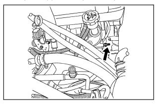
The remote negative (-) terminal is a stud located on the right front passenger side of the engine, where the negative battery cable attaches. See *Engine Compartment Overview on page 5-14*.
