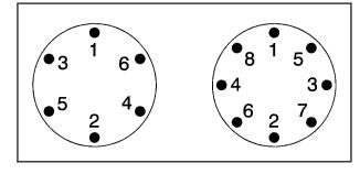
Tighten the nuts firmly in a crisscross sequence as shown by turning the wheel wrench clockwise.
