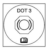
The brake master cylinder reservoir is filled with DOT-3 brake fluid. See Engine Compartment Overview on page 5-14 for the location of the reservoir.
