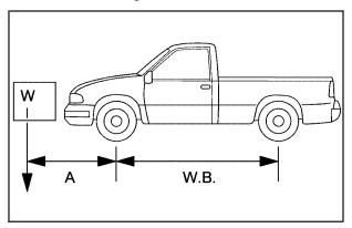
(W x (A + W.B.)) /W.B.= Weight the accessory is adding to the front axle.
