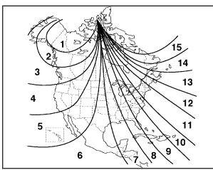
Press and hold the on/off button until a Z and a zone number appears in the display. The compass is now in zone mode.  Keep pressing the on/off button until the desired zone number appears in the display. Release the button. After approximately four seconds of inactivity, the new zone number will be locked in and the compass/temperature display will return.
