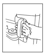
To open a rear access door from the inside, the front door must be opened first. Then, use the handle located on the inside of the rear access door to open.
