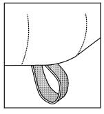
Pull up on the front of the seat cushion while pulling down on the release strap, located under the seat cushion.
