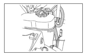
The coolant level should be at or above the FULL COLD mark. If it is not, you may have a leak at the pressure cap or in the radiator hoses, heater hoses, radiator, water pump, or somewhere else in the cooling system.
