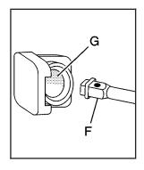
Insert the hoist end (F) through the hole (G) in the rear bumper and onto the hoist shaft.
