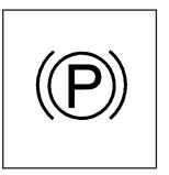
A parking brake symbol is located next to the N (NEUTRAL) symbol as a reminder to set the parking brake before shifting the transfer case in Neutral.
