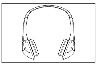
The RSE includes two 2-channel wireless headphones that are dedicated to this system. Channel 1 is dedicated to the video screen, while Channel 2 is dedicated to RSA selections. These headphones can used to listen to the radio, CDs, DVDs, MP3s, DVDAs, any auxiliary source connected to A/V jacks, or the auxiliary input jack, if the vehicle has this feature. The wireless headphones have an On/Off button, channel 1/2 switch, and a volume control.
