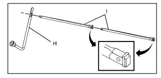
Attach the wheel wrench (H) and extensions (I) together, as shown.
