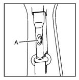
push down on the release button (A) and move the height adjuster to the desired position.
