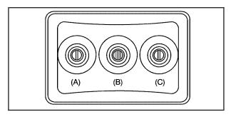
The A/V jacks, located on the rear of the floor console, allow audio or video signals to be connected from an auxiliary device such as a camcorder or a video game unit to the RSE system. Adapter connectors or cables (not included) may be required to connect the auxiliary device to the A/V jacks. Refer to the manufacturer's instructions for proper usage.
