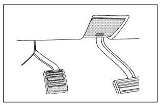
To release the parking brake, hold the regular brake pedal down. Then pull the bottom edge of the lever, with the parking brake symbol and located above the parking brake pedal.
