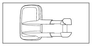
If the vehicle has trailer towing type mirrors, they can be adjusted so you can have a clear view of the objects behind you. Manually pull out the mirror head to extend it for better visibility when towing a trailer.
