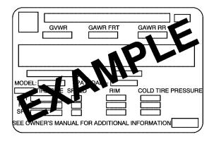
A vehicle specific Certification/Tire label is found on the rear edge of the driver's door. The label shows the size of your vehicle's original tires and the inflation pressures needed to obtain the gross weight capacity of your vehicle. This is called Gross Vehicle Weight Rating (GVWR).
