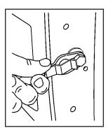
Raise the tailgate slightly and release both retaining cable clips. To release the retaining cable clips, lift the cable so it points straight out. Lift the clip over the bolt, and push the cable forward then rotate down.
