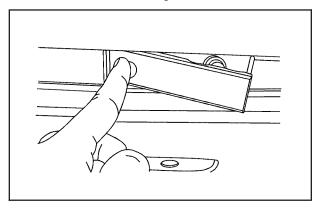
To open, press and hold the driver's side of the handle in and pull out on the exposed portion of the handle.
