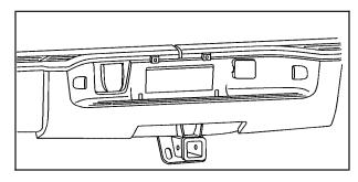
For vehicles equipped with heavy duty trailering, the harness is connected to a bracket on the hitch platform. The seven-wire harness contains the following trailer circuits:
