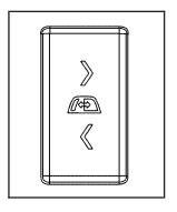
On vehicles with a power sliding rear window, the switch is located in the overhead console.
