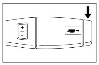
If your vehicle has an Allison or Hydra-Matic<sup>®</sup> 6-speed automatic transmission<sup>®</sup>, it has a tow/haul mode. The tow/haul mode adjusts the transmission shift pattern to reduce shift cycling, providing increased performance, vehicle control, and transmission cooling when towing or hauling heavy loads.
