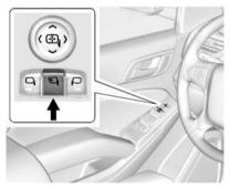
To adjust power folding mirrors, if equipped:
