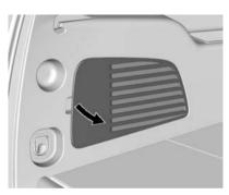
The rear compartment fuse block is behind the access panel on the left side of the compartment.
