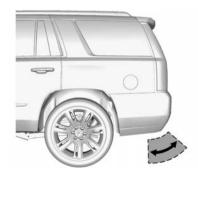
To operate, kick your foot straight up in one swift motion under the center of the rear bumper, then pull it back.
