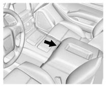
Pull the handle and lift to access the console. There are auxiliary jacks, USB ports, an accessory power outlet, tote compartment, device holder, and SD card reader inside.
