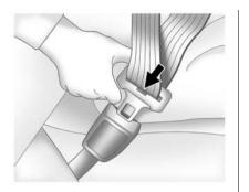
3. Push the latch plate into the buckle until it clicks. If you find that the latch plate will not go fully into the buckle, see if you are using the correct buckle.
