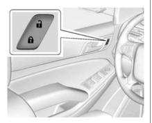
**(Lock):** Press to lock the doors. **(Unlock):** Press to unlock the doors.
