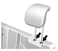
2. Press the buttons on the head restraint posts, and pull up on the head restraint.
