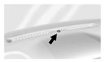
The solar sensor monitors the solar heat. Do not cover the solar sensor or the system will not work properly. There is also an exterior temperature sensor behind the front grille. This sensor reads the outside air temperature and helps maintain the temperature inside the vehicle. Any cover on the front of the vehicle, including a snowplow, could cause a false reading in the displayed temperature.
