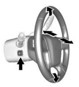
To adjust the power tilt and telescope steering wheel, if equipped:
