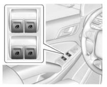
The power windows work when the ignition is in ON/RUN or ACC/ ACCESSORY, or in Retained Accessory Power (RAP). See Retained Accessory Power (RAP) on page 9-27. If equipped, the front and rear windows have an express-down feature. The front windows have an express-up feature. See *Windows on page 2-33* and *Power Windows on page 2-33*.
