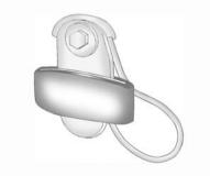
Remove the guide from its storage clip on the interior trim next to the outboard seatback.
