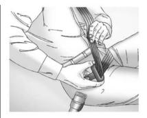
For front seating positions, if the webbing locks in the latch plate before it reaches the buckle, tilt the latch plate flat to unlock.
