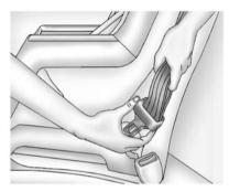
2. Pick up the latch plate, and run the lap and shoulder portions of the vehicle's safety belt through or around the restraint. The child restraint instructions will show you how.
