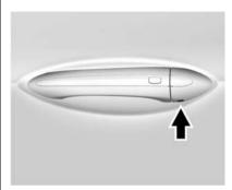
To access the key cylinder, insert the key into slot on the bottom of the door handle and pry cover off. Replace cover when done by snapping on tabs.
