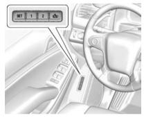
If equipped, the SET, "1," "2," and (Exit) buttons on the driver door are used to manually store and recall memory settings for the driver seat, outside mirrors, power tilt and telescoping steering column (if equipped), and adjustable pedals (if equipped).
