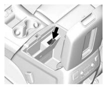
5. Place the new transmitter in the transmitter pocket/insert.
