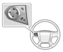
(**On/Off):** Press to turn the system on or off. A white indicator comes on in the instrument cluster.
