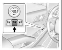
To adjust power folding mirrors, if equipped:
