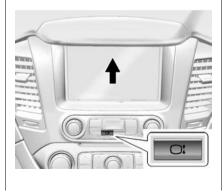
If equipped with storage behind the radio, press and hold  $\bigcirc_{\downarrow}^{\uparrow}$  to open. There is a USB port inside. See the infotainment manual.
