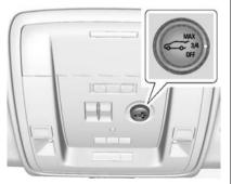
If equipped, the switch is on the overhead console. The vehicle must be in P (Park).
