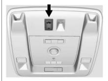
It is recommended that the intrusion and inclination sensors be deactivated if pets are left in the vehicle or the vehicle is being transported. With the vehicle off, press in the front overhead console to turn off the feature.
