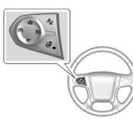
S: Press to turn the system on or off. The indicator light is white when cruise control is on and turns off when cruise control is off.
