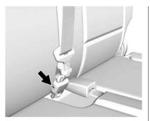
Disconnect the rear safety belt mini-latch, using a key in the slot on the mini-buckle, and let the belt retract into the headliner. Stow the mini-latch in the holder in the headliner.
