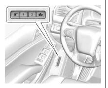
If equipped, the SET, "1," "2," and (Exit) buttons on the driver door are used to manually save and recall memory settings for the driver seat, outside mirrors, power tilt and telescoping steering column (if equipped), and adjustable pedals (if equipped).
