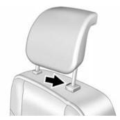
The third row seat head restraint can be lowered for better visibility when the rear seat is unoccupied.
