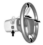
To adjust the power tilt and telescope steering wheel, if equipped:
