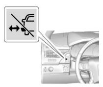
If equipped, the power assist steps will deploy when the door is opened and automatically retract three seconds after the door is closed. The power assist steps will retract immediately if the vehicle starts moving.
