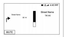
Press the button below the MUTE screen button to mute the navigation directions. The previous audio selection will play. The MUTE screen button will change to UNMUTE. Press the button below UNMUTE to enable the navigation directions again.
