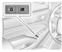
Press i to activate the safety locks on the rear doors. The indicator light comes on when activated.
