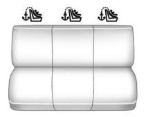
Third Row Seat (Top Tether Anchor): Seating positions with top tether anchors.
