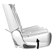
2. Lift the lever, on the outboard side of the seat, to release the seatback.
