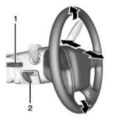
To adjust the tilt and telescope steering wheel, if equipped:
