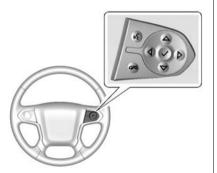
$\triangle$  or  $\nabla$ : Press to move up or down in a list. In the main view, you can press up and down to move between different info app pages.  $\triangleleft$  or  $\triangleright$ : Press to move between the interactive display zones in the cluster.
