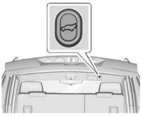
Press any liftgate button, the touch pad, or  $\cancel{42}$  on the RKE transmitter while the liftgate is moving to stop it. Pressing again restarts the operation in the reverse direction. The touch pad on the liftgate handle cannot be used to close the liftgate. Do not manually force the liftgate to open or close during a power cycle.
