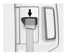
Push down on the release button to move the height adjuster to the desired position.
