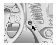
Vehicles with Keyless Access have pushbutton starting.
