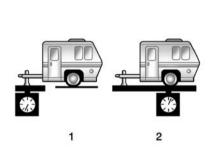
Trailer tongue weight (1) should be 10 % to 15 % of the loaded trailer weight (2) up to the maximums for vehicle series and hitch type.
