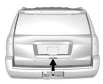
To open the liftgate, press a on the power door lock switch or press a on the Remote Keyless Entry (RKE) transmitter twice to unlock all doors.
