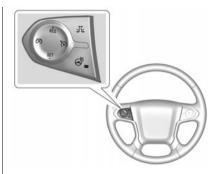
(**On/Off):** Press to turn the system on or off. The indicator turns white on the instrument cluster when ACC is turned on.
