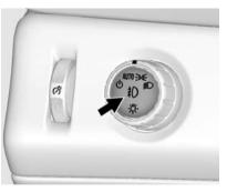
If equipped with fog lamps, the button is on the exterior lamp control, to the left of the steering column.
