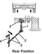
**Rear Tire Flat:** If the flat tire is on a rear tire of the vehicle, use the jack handle (2) and both jack handle extensions (3). Attach the wheel wrench (4) to the jack handle extensions (3). Attach the jack handle (2) to the jack (1). Use the jacking pad (5) provided on the rear axle. Turn the wheel wrench (4) clockwise to raise the vehicle. Raise the vehicle far enough off the ground so there is enough room for the spare tire to clear the ground.
