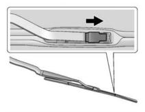
2. Lift up on the latch in the middle of the wiper blade where the wiper arm attaches.
