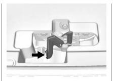
2. Go to the front of the vehicle to find the secondary hood release. The handle is under the front edge of the hood near the center. Push the handle to the right and at the same time raise the hood. Before closing the hood, be sure all the filler caps are on properly. Then bring the hood from full open to within 15 cm (6 in) from the closed position, pause, and push the front center of the hood with a swift, firm motion to fully close the hood.
