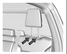
Press both buttons on the head restraint or headrest posts at the same time, and pull up on the head restraint or headrest.
