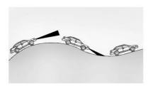
Do not use ACC when driving on steep hills or when towing a trailer. ACC will not detect a vehicle in the lane while driving on steep hills. If the brakes are applied, ACC disengages.
