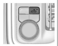
The cargo lamps provide more light in the cargo area or on the sides of the vehicle, if needed. The lamps inside the pickup box, in the tailgate handle, for the hitch, and/or the cargo mirror lamps also turn on, if equipped.
