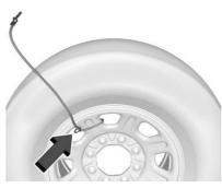
9. If equipped with a spare tire cable remove the cable from the spare tire by passing the clip through the looped end of the cable.
