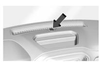
The solar sensor, on top of the instrument panel near the windshield, monitors the solar heat.
