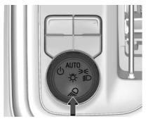
If equipped, task lighting projects light from the outside mirrors away from the vehicle. While the vehicle is parked, press  $\mathcal{R}$  to select one of the following options:
