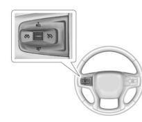
(5): Press to turn the system on or off. The indicator turns white on the instrument cluster when ACC is turned on.
