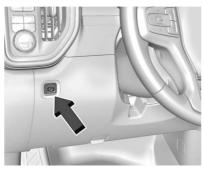
The vehicle has an Electric Parking Brake (EPB). The EPB can always be activated, even if the ignition is off. To prevent draining the battery, avoid repeated cycles of the EPB when the engine is not running.
