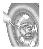
2. If the vehicle has wheel nut caps, loosen them by turning the wheel wrench counterclockwise.
