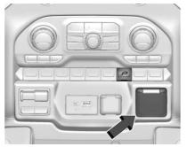
In Cab Power Outlet and DC/AC Switch
