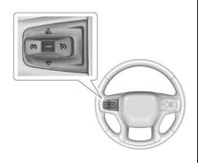
: Press to turn cruise control on or off. A white indicator comes on or off in the instrument cluster.
