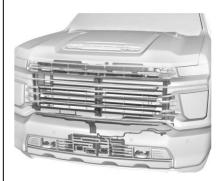
The vehicle may have a shutter system designed to help increase fuel economy. Keep the shutter system clean for proper operation.
